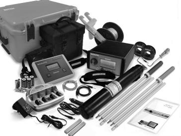
By measuring the voltage differential between the test probes, the detector unit is able to direct the operator to the location of the leak.
