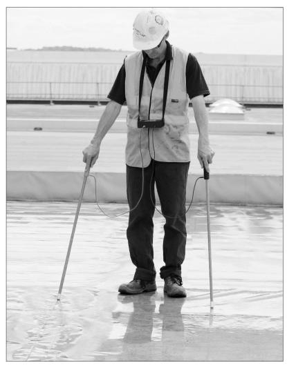
attached to the trace wire. The clip must be positioned to clamp together the free end of the trace wire to the section of wire emerging from the reel to complete the loop around the test area. The generator unit should now be switched on.
