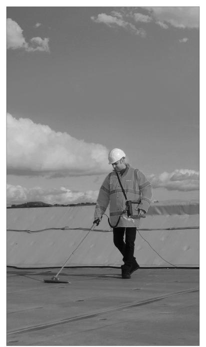
A suitable point on the structure should be identified as an earth connection for the earth lead of the Dry Roof Pro'.
